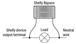
Connect the Shelly Bypass in parallel to the load as shown on the diagram above.
